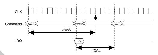
Note: Internal auto-precharge starts at the timing indicated by " ". and an interval of tRAS (/RAS) is required between previous active (ACT) command and internal precharge " ". ".
