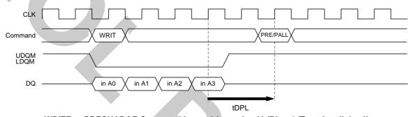
WRITE to PRECHARGE Command Interval (same bank) (BL = 4 (To write all data))
